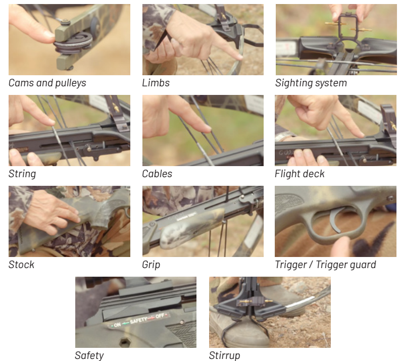
Picture 5.7 Components of a compound crossbow
