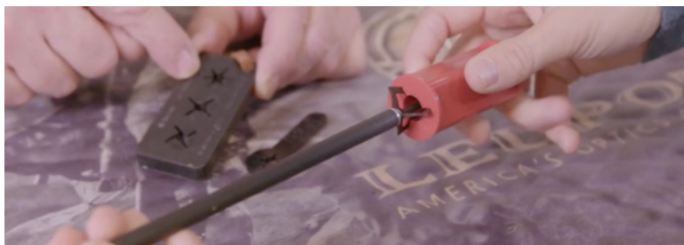
Picture 5.12 Specially designed tools to unscrew the broadheads
