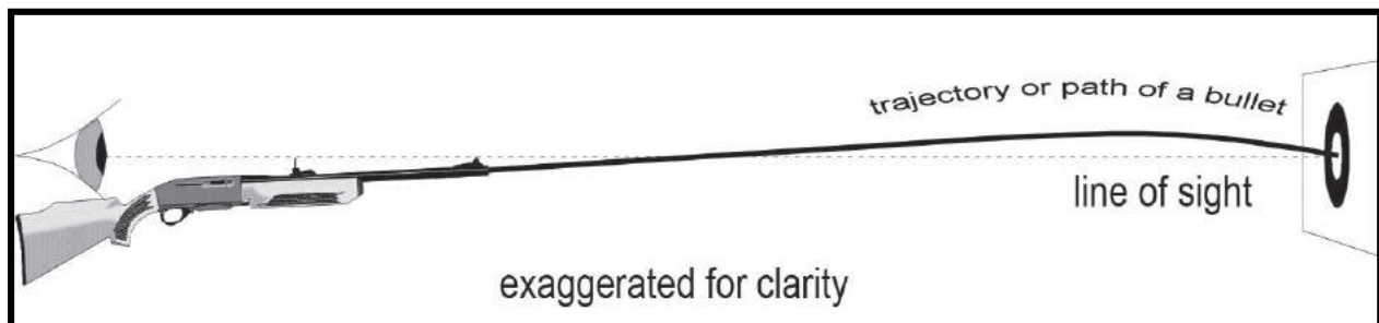
Figure 39. Trajectory of a Bullet
