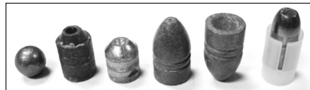
Round ball, conical bullet, lubricated conical, bullet, Minié bullet (front and back views), and sabot bullet
