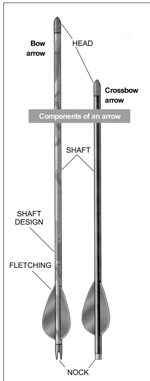
An arrow that has the right amount of stiffness for your bow or crossbow will lose the least energy, i.e. fly the best and have the flattest trajectory. Stiffness depends on the material the arrow is made of and the arrow's length and weight. Shooting arrows that are lighter or shorter than those recommended by the manufacturer can be dangerous. That is why it is important to always use the arrows that are recommended for your particular weapon.
