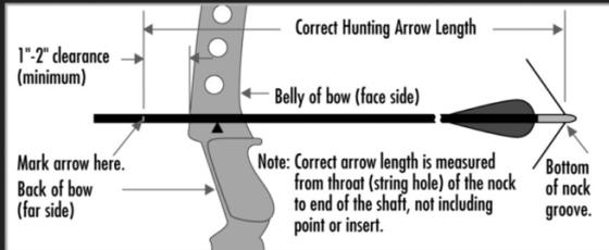
**Bow Draw Length.** Draw length is measured at full draw from the bottom of the nock groove to the back (far side) of the bow. Actual arrow length and draw length are only the same if the end of the arrow shaft is even with the back of the bow (far side) at full draw.
