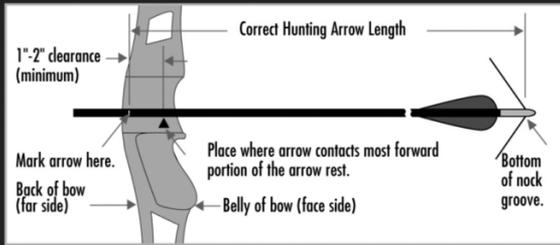
**Bows without cut-out window** (which will not allow a fixed blade broadhead to be drawn past the back of the bow). The Correct Hunting Arrow Length for bows without a cut-out sight window is determined by drawing back an extra-long arrow to full draw, and having someone mark the arrow one to two inches in front of the handle.
