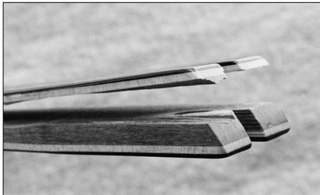
Typical example of delamination
